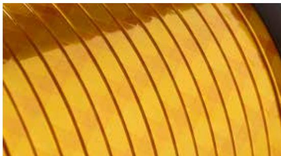
flat aluminium wire insulated with 2 layers SynTherm® H, in opposite directions, 25 % overlap
