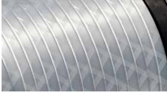
flat enameled aluminium wire insulated with 2 layers SynTherm® P, in opposite directions, 20 % overlap
