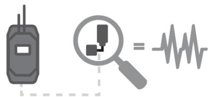
CLOUD ID is a technology that allows gateways to automatically recognize sensors and configure a cloud dashboard. This technology is found in many of our wireless sensor nodes that measure vibration, differential pressure, temperature and humidity, tank level, and more.
