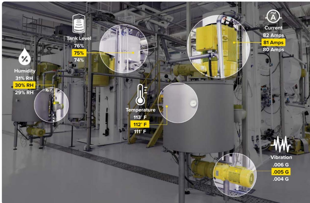
Use the simple binding process to bind sensor nodes to a gateway, and monitor tank level, ambient temperature and humidity, and the health of rotating machines and pressurized systems.
