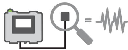
SNAP ID enables our gateways to automatically identify a wired sensor, understand what data it is able to share, and present the data in easy-to-understand units such as pressure and current. This technology is found in many of our wired sensors that can monitor vibration, temperature, humidity, current, pressure, level, and dew point.
