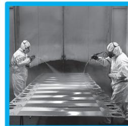
Dye Penetrant Test
