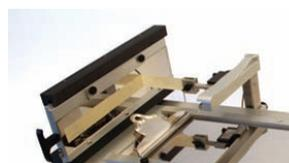
The 90 degree peel fixture is an ideal accessory for adhesive materials. Also available with a heated option.
