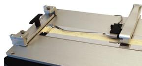
The 180 degree peel arm for peel testing is included with all FP-2260 units.
