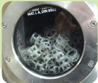
Filling material in the vapour scrubber
