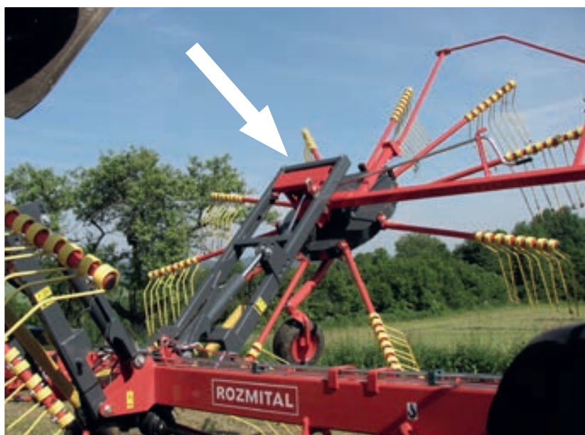
Automatic return of rotors to transport position when folding the arms
