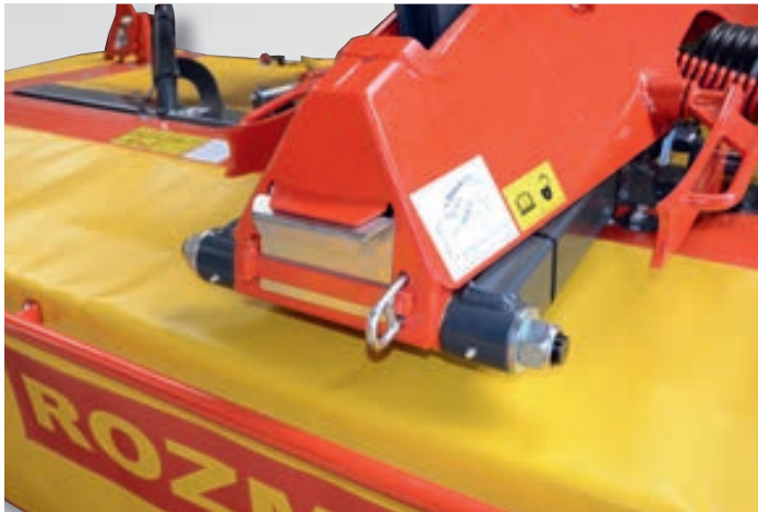
Lever for blade quick release and spare blades storage compartment.
