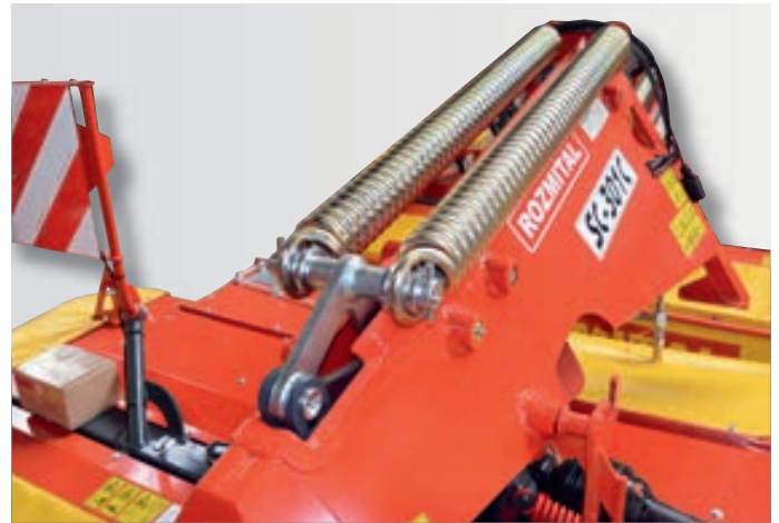
Cutterbar flotation by using springs.
