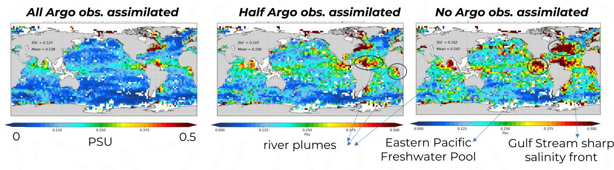
Significant degradation of the ocean analysis and forecast quality when reducing the number of assimilated Argo observations.
