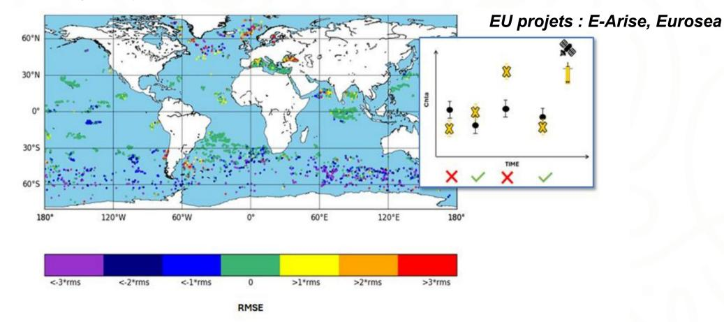
**Figure 4: Schematic information available through the webtool dashboard.** Map of BGC-Argo and satellite matchups. The colour of the dots corresponds to the thresholds of the difference between satellite and BGC-Argo surface data. And on the right panel, Chla timeseries for a particular float, and comparison with satellite observations. The error bars correspond to the uncertainty and allow to identify suspicious profiles
