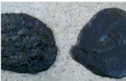
Fermentation substrate before and after disintegration with Impra
