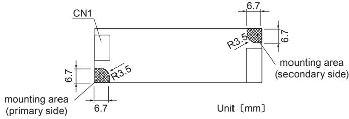
■ The mounting area (primary side) must be insulated from areas that user accessible parts of the final product, so if the enclosure is metal and the mounting components and spacers are metal, be careful to insulate them.
