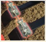
The Spring-Board tines can work individually but the levelling effect is increased with the addition of the HE-VA optional transverse locking system, to convert the individual springs into a complete "board" for full width action. This locking system is easy to mount / dismount tine by tine.
