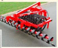
4 m Spring-Board for 1.65 m Front-Pakker has as standard mechanical change-over into a transport width of 2.85 m.
