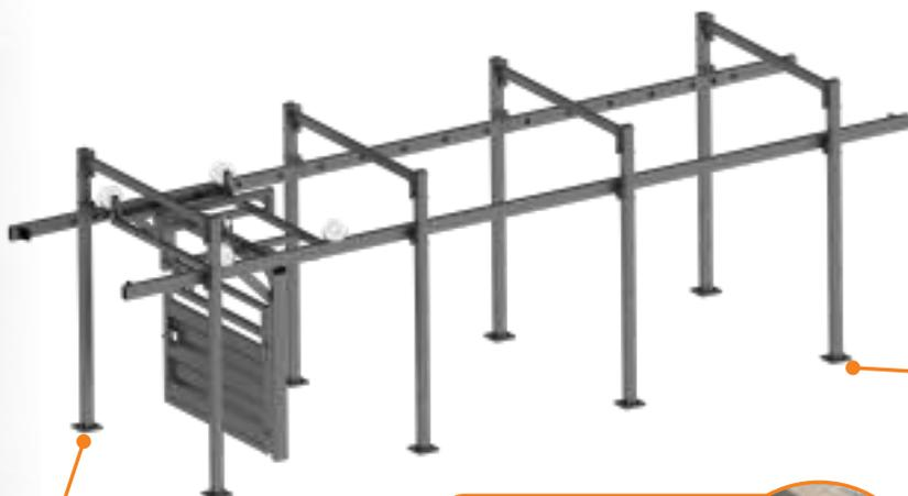
Poteaux et traverses en tube 100x100x4mm
