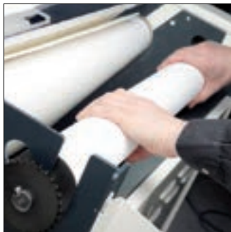
Moulding belts Ultra-fast change of belts without disassembling the machine
