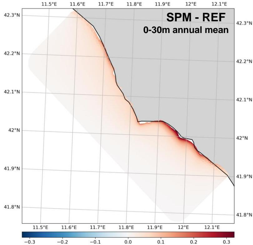
**Light Extinction is higher in SPM experiment over all the domain → due to suspended sediments in the water column**
