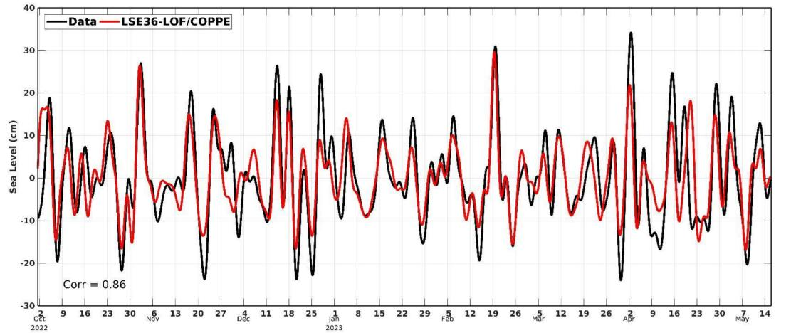
Sea level variations inside GB: The coastal Delft3D model nested within the LSE36-LOF/COPPE model (red) more closely matches observed data than the coastal model forced only by the TPXO9 tide model (blue). The use of LSE36-LOF/COPPE model at the oceanic open boundary allows oceanic subinertial processes to propagate into the coastal domain, reducing the error.
