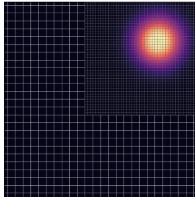
The Spall and Holland (1991) baroclinic vortex test-case (SST) replicated with NEMO-AGRIF (the zoom uses a refinement factor of 3; from <https://sites.nemo-ocean.io/user-guide/zooms.html>).
