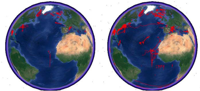
FIGURE 1 | Development of the glider activity over the past decade. Gliders tracks of past deployments (left) until December 2009 (OceanObs'09) and (right) until October 2018 (OceanObs'19 submissions), as can be viewed using google-earth.
