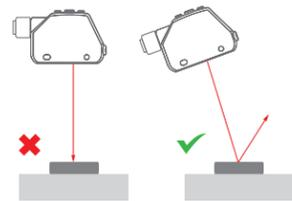
TIP: Change sensor orientation by a few degrees for more reliable detection of shiny objects
