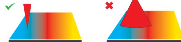
A small beam spot is ideal for precise profiling of small features
