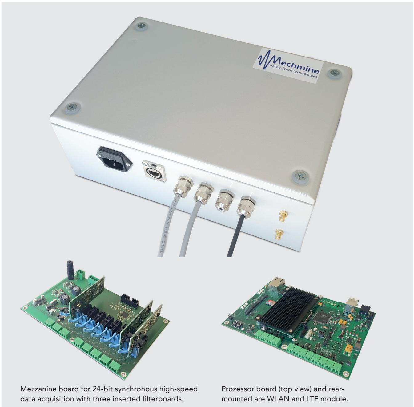
Mezzanine board for 24-bit synchronous high-speed data acquisition with three inserted filterboards.
