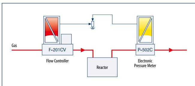
The control valve of the EL-FLOW F-201CV Mass Flow Controller (MFC) forms a closed loop pressure control system with the EL-PRESS P-502C Pressure Transducer: the Mass Flow Meter of the MFC measures the required flow rate to maintain the set pressure level. The setpoint voltage divider enables the user to adjust the maximum flow to build up desired pressure levels. Restriction of the maximum flow may for safety reasons be important in certain processes.
