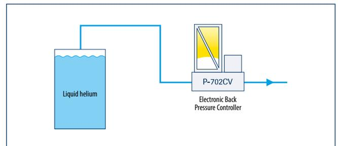
Superconducting coils, which are used to generate magnetic fields, are cooled by liquid helium. Depending on the temperature exchange gaseous helium should be vented. With a manually controlled outlet the variation of the atmospheric pressure disturbs the magnetic field. By using an EL-PRESS P-702CV Back Pressure Controller the pressure for the superconducting coils is kept constant, thus eliminating the negative effects of atmospheric pressure variations.
