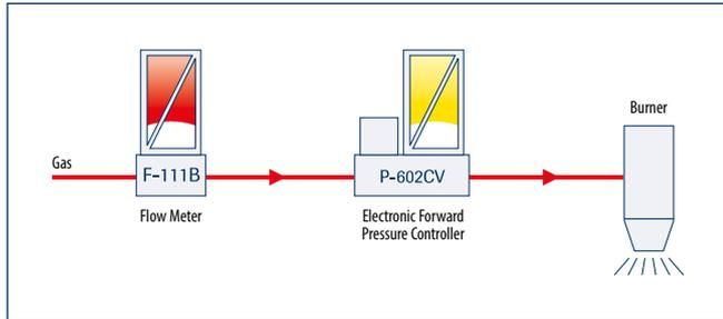
This arrangement of an EL-FLOW Mass Flow Meter with, in series, an EL-PRESS Forward Pressure Controller is used in burner test applications, or tests to check the inlet pressure dependence of the capacity of mechanical pressure regulators, or the tolerance on the bore of orifices, etc.
