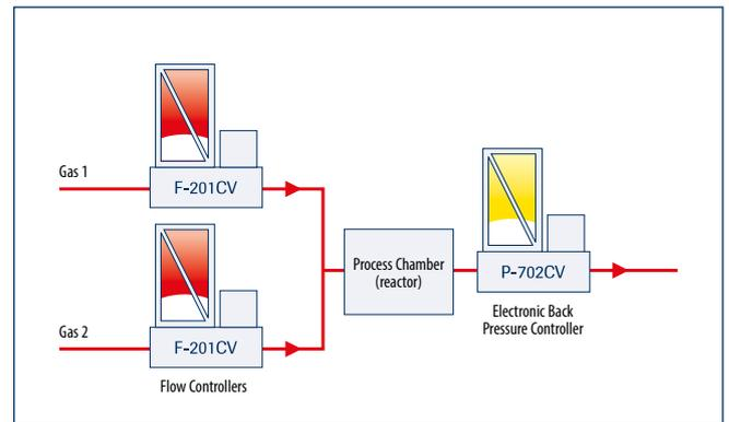
A gas mixture is formed by EL-FLOW Mass Flow Controllers. In a process chamber the effect of the catalyst on certain reactions is tested. The pressure in the process chamber is controlled to the desired level by means of an EL-PRESS Back Pressure Controller, independent of the total flow and/or the composition of the mixture.
